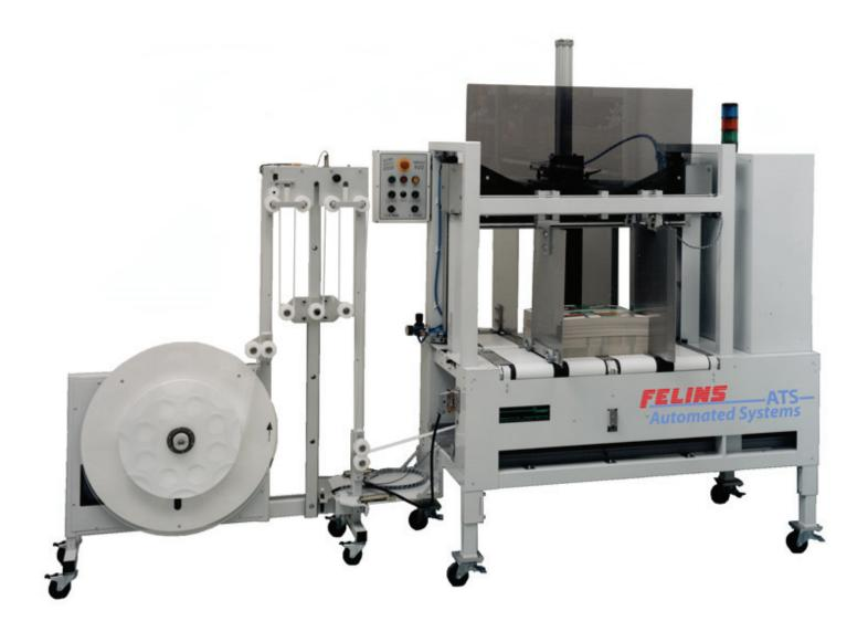
The fully automatic Transit ASX is specifically designed for banding high-gloss color graphic corrugated materials. A large product opening and long rolls of material make this machine ideal for corrugated applications. The special FWG 210-30-1300 banding material will not damage the edges of the top and bottom of the stack, yet will tightly hold the bundle for transport. This system is used in-line as part of the packaging procedure to hold counts and to prevent scuffing.
